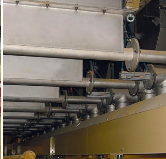
Dosierschnecken DS Differentialwaage | Metering screws DS differential scale
